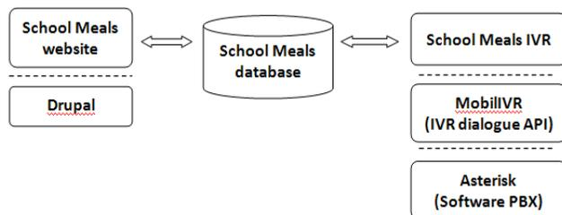
**Figure 3. System architecture.**
